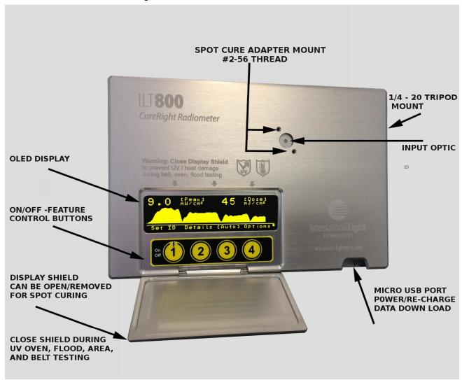
(Note: the ILT800 accepts two #2-56 screws for mounting spot cure adapters. Adapters allow the user to assure an accurate/repeatable working distance is used each time. Small changes in alignment and distance can cause significant changes in results when measuring spot cure sources and LED's.)
