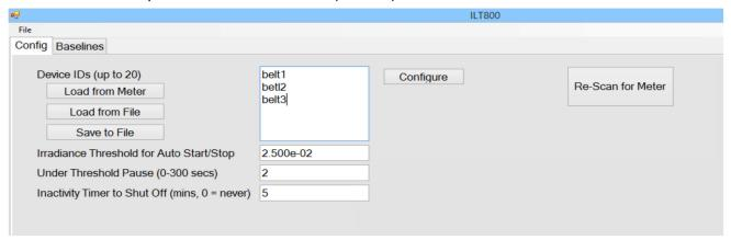
The "Configure" Button will load the meter with the parameters entered.
